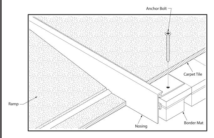
**NOTE:** Nosing to be used at the edge of the floor to create a step or along the side of a ramp.
